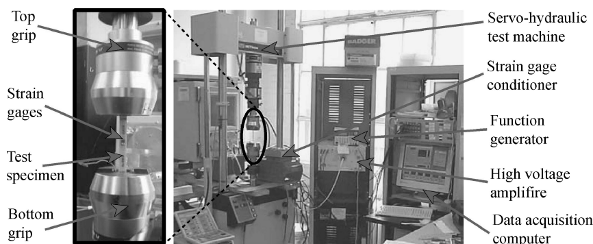
Fig. 12 Mechanical fatigue test setup with servohydraulic tensile testing machine.
